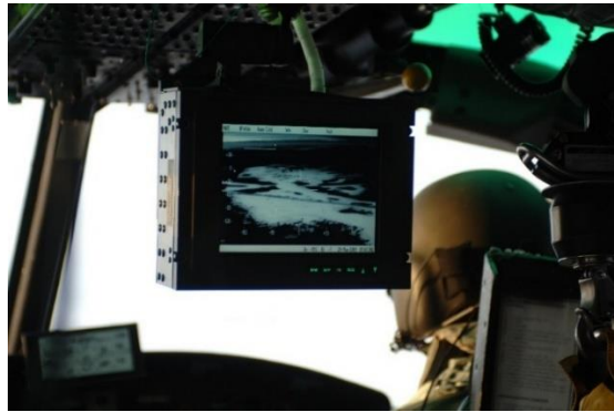
Figure 9: A Forward-looking Infrared (FLIR) system on a U.S. Air Force helicopter during search and rescue operation
