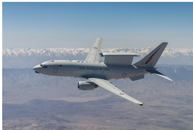
Figure 27: A Royal Australian Air Force E-7A Wedgetail. It provides airborne surveillance and early warning systems.
